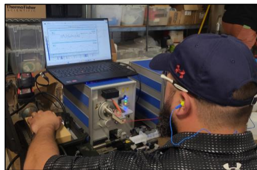
Figure 6. Implementation of a rapid screening method for PFAS detection, direct analysis in real-time (DART).
